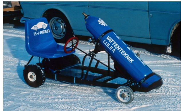
Fig. 2 A small go-kart vehicle (icy rider) which was built and used to test the theoretical model
