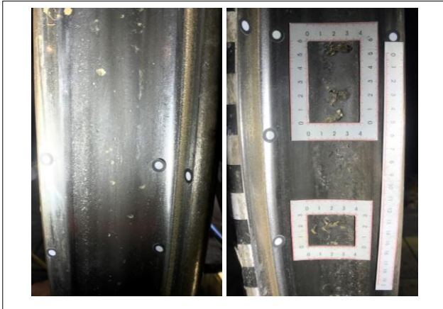
Figure 1 – Left: Section of the tread surface of the less damaged wheel. Rounded indentations and some minor wear are visible. Right: Section of the tread surface of the damaged wheel where two of the main RCF clusters are located.
