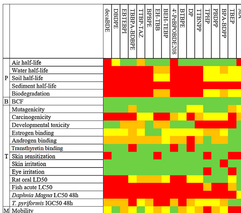
Figure 2. Heat map of the 17 flame retardants where red indicates that a hazard criterion has been met, orange and yellow indicate high and moderate hazard level, and green indicates that the chemical has properties fulfilled a set safe level (SI Section 2). Thresholds for the four categories of each criterion is listed in SI Table S3.
