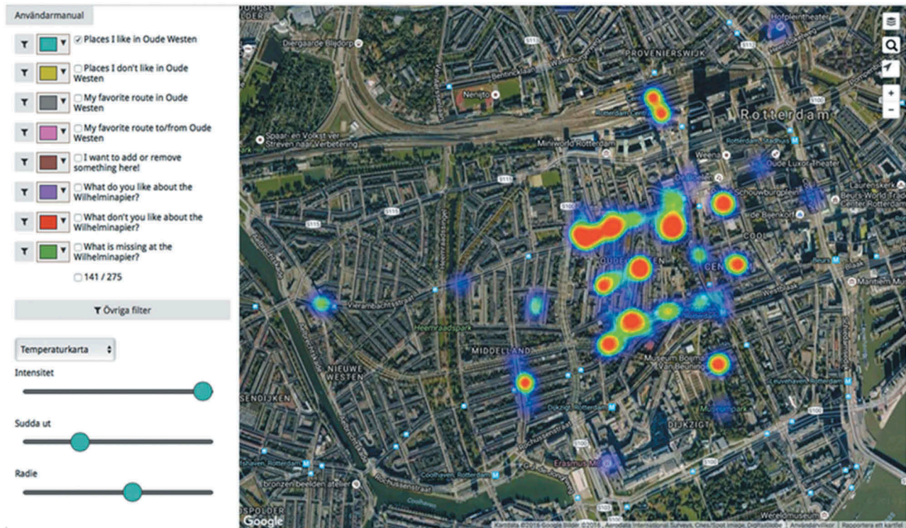
Figure 10. Example of spatial visualization of perceptions of places as a heatmap, using the software Maptionnaire. Surveys collected from citizens in the street in a Rotterdam district were translated into markers of places they liked and disliked and were digitally analysed, where each such marker contains additional qualitative data.
