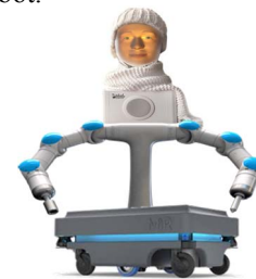
Fig. 4. Hybrid Concept of Embodied Automation combining (top-down) Furhat Robotics, SciMotion Robotics and MiR Robotics
