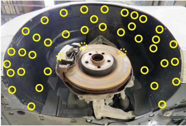
Figure 8: Wheelhouse pressure sensor locations. Front left wheelhouse.
