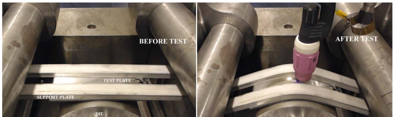
Figure 2. Test set up for the Vareststraint test.
