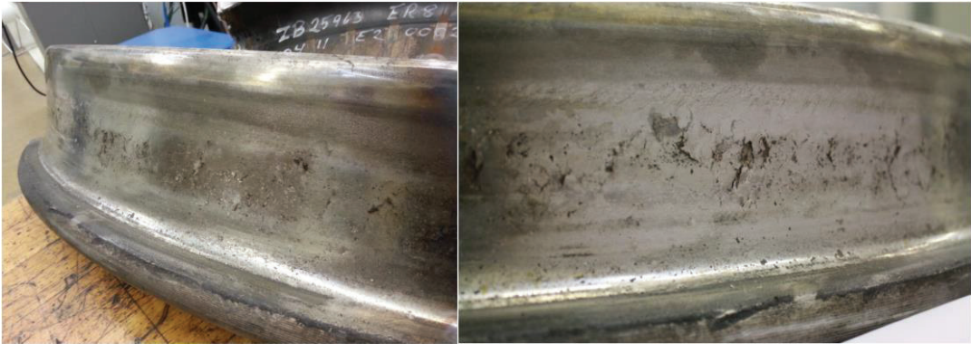
Figure 31. Wheel treads with RCF1 and RCF3 damage bands.
