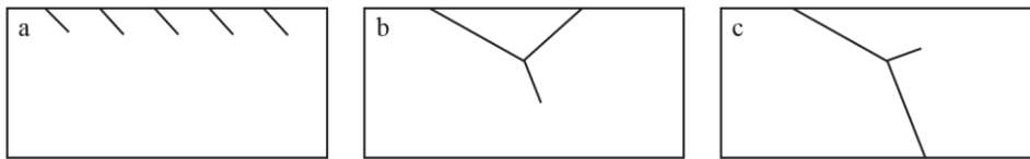
Figure 4. Schematic showing three levels of severity of RCF cracks on rail surface: (a) small cracks, (b) spalling, and (c) risk for rail break. (Longitudinal section) [27]
