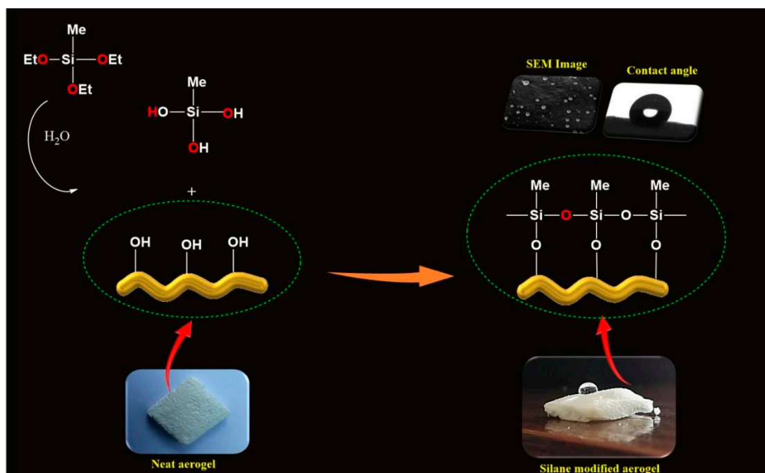
Figure 3. The strategy for the formation of polysiloxane particles during the silane modification of CNF aerogels.
