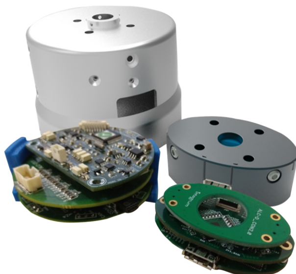
Figure 8.1: Representation of the Artificial Limb Controller versions: ALC-transhumeral (left) and ALC-transradial (right). Such system provide a clinically viable solution for the control of upper limb prostheses, as well as a research platform for further investigations on prosthesis usage and training, machine learning techniques and neural stimulation paradigms.
