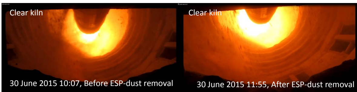
Figure 24: Before removal of ESP dust (left) and after removal of ESP dust (right) from 30 June 2015.
