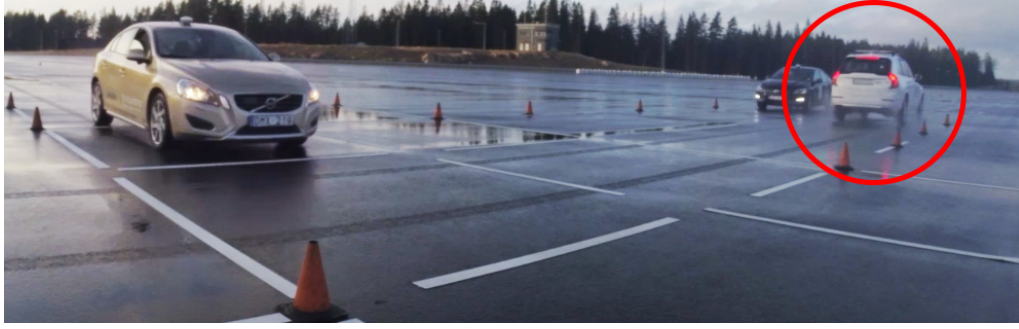
Figure 6.11: Photo from an experimental run. The white vehicle applies the friction-brake immediately after leaving the intersection (marked with white lines).
