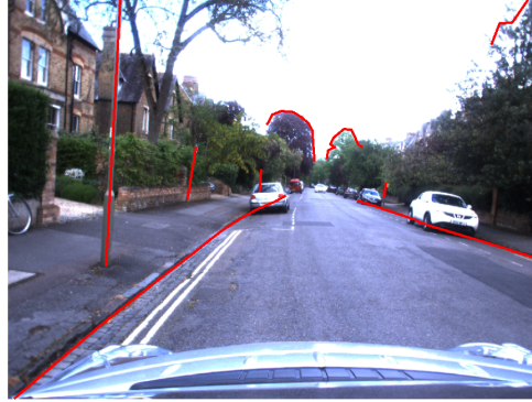
Figure 3.1: Illustration of the method in Paper IV. Any given pose may be evaluated by how well the semantically labelled structure projects down into the given pose. Only the semantic 3D curves are shown (poles, road edge, vegetation-sky contour). 3D points (not shown) were used as well.
