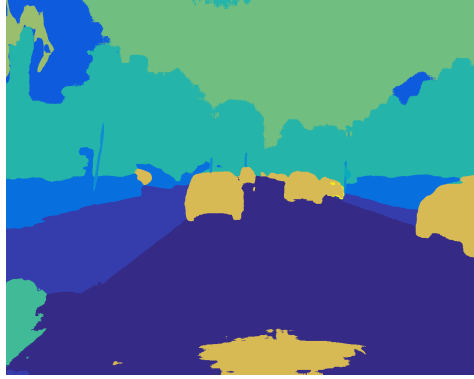
Figure 2: A typical example of a pixelwise semantic labelling of a picture from the Oxford Robotcar dataset.
