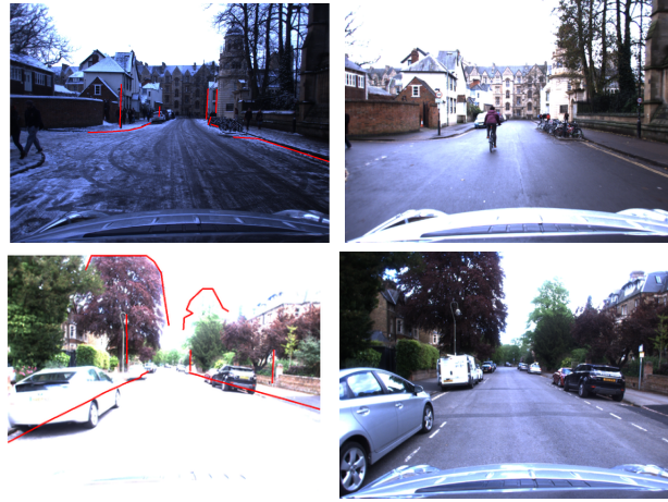
Figure 1: Two examples of successfully localized pictures. In the left column, the query images are shown together with the reprojection of the 3D curves corresponding to road edges and poles. The images on the right show approximately the same location as seen in the mapping sequences. Note that our baseline method based on LIFT features failed to obtain consistent 2D-3D matches.
