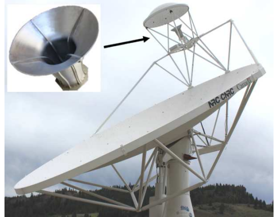
Fig. 1. QRFH (top left) installed on DVA-1, seen just below the sub-reflector.
