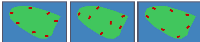
Figure 24: Layouts from pure view optimization. From left to right, the initial layout was hexagonal, principal line, and coastal, respectively
