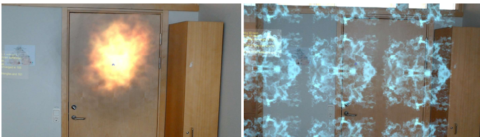
Figure 5: Problem data represented by holograms. Left : Source (fire ball) placed in room. Right : Zero value boundary conditions (ice patches) on wall.
