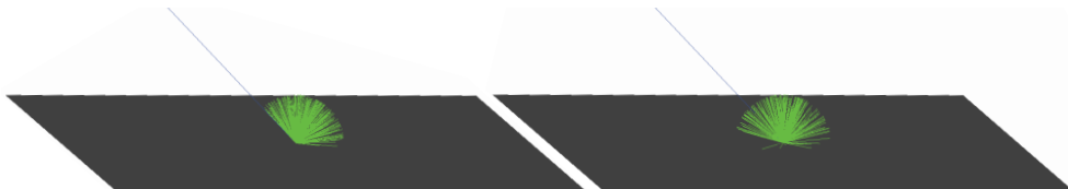
Figure 4.15: Scattering from a surface coated with Vantablack S-VIS (left) and a surface coated with an ideal Lambertian scatterer (right).
