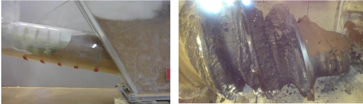
Figure 3.8. Left: Cold flow model showing bed material pushed into the fuel feeding screw. Source: Claes Breitholtz, Valmet AB. Right: Feeding screw used in the GoBiGas plant, exhibiting mainly graphite-like deposits. From [15].
