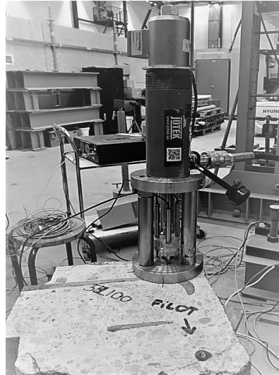
Figure 3.8: Pull-out test set-up
