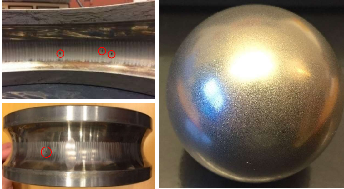
Figure 130. Electrical fluting damage on bearing surfaces on the outer raceway (left-top), inner raceway (left-bottom) and micro-craters (electrical pitting) on the ball (right), giving it a satin, frosty or a matte like finish.
