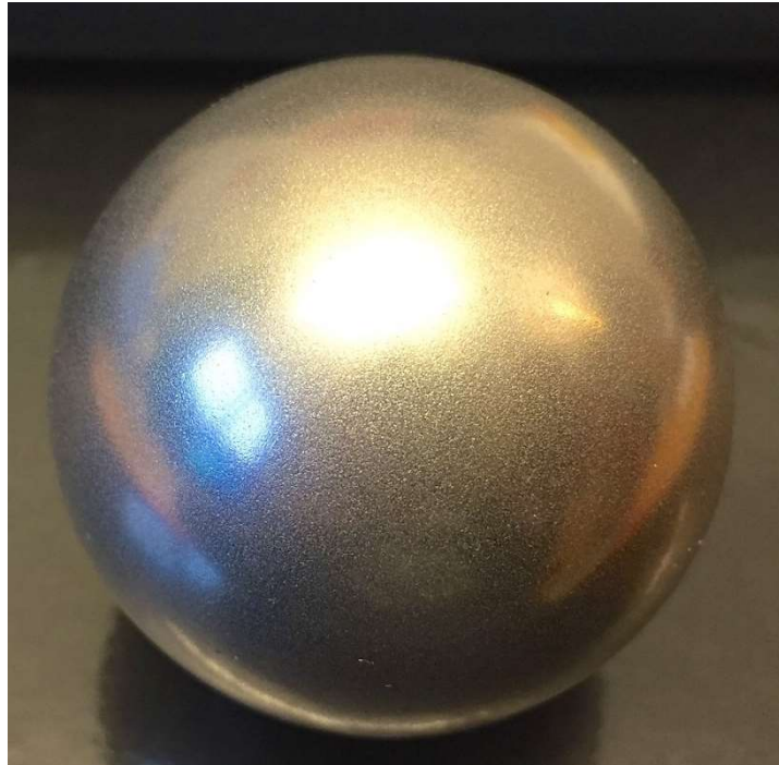
Figure 6. Damages on the bearing's ball due to electrical discharges form micro-crater on the ball, giving it a matte finish.
