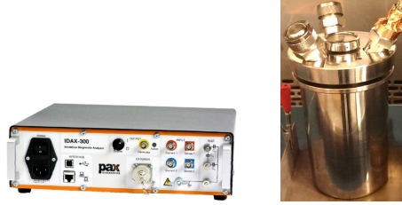
Figure 32. IDAX 300 [42] (left), used in FDS and Tettex oil test cell (right).
