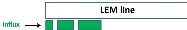
Figure 1.6: Order of joining of the LEM segments to the input boundary on the basis of flux
