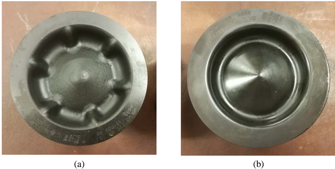
Figure 3-2 The geometries of the tested a) 6-wave piston and b) standard \omega -bowl piston.
