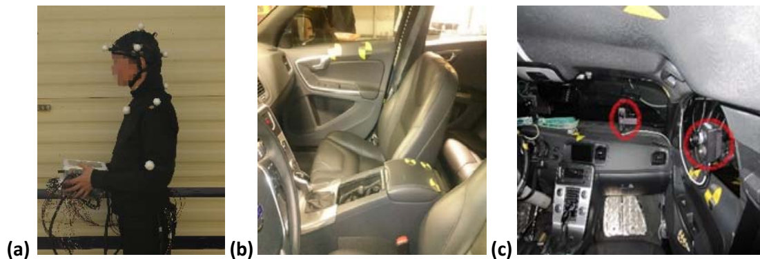
Fig. 1. (a) Volunteer prepared for test, (b) passenger seat position, (c) interior of test vehicle presenting side and front cameras, foot plates for the passengers and photo targets.
