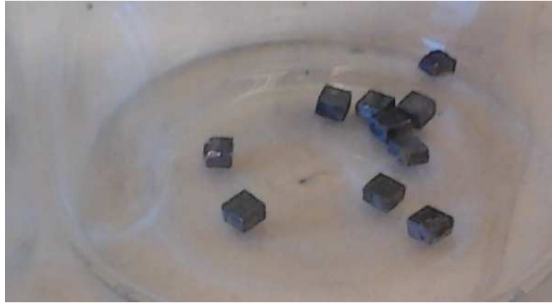
Figure 2.14: The size (1.6 mm \times 1.6 mm \times 1 mm) of the thermoelectric legs in the harvester. The material in this picture is Ba 8 Ga 16 Ge 30 .
