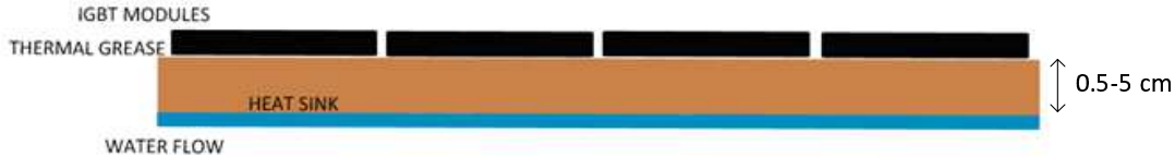
Figure 6.2: Power stack structure.
