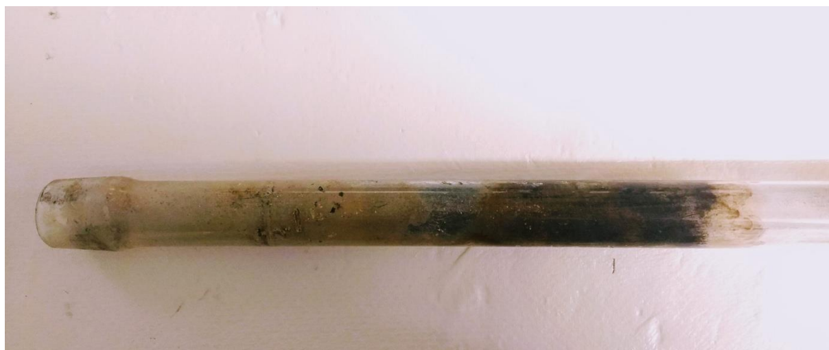
Figure 20: The internal section of the quartz tube covered with the organic by-product.
