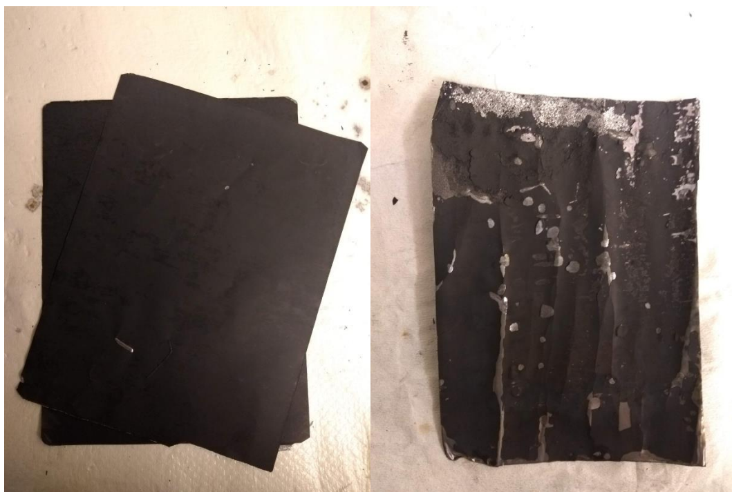
Figure 21: Comparison of an untreated cathode (left) with one treated at 700°C for 90 minutes (right).
