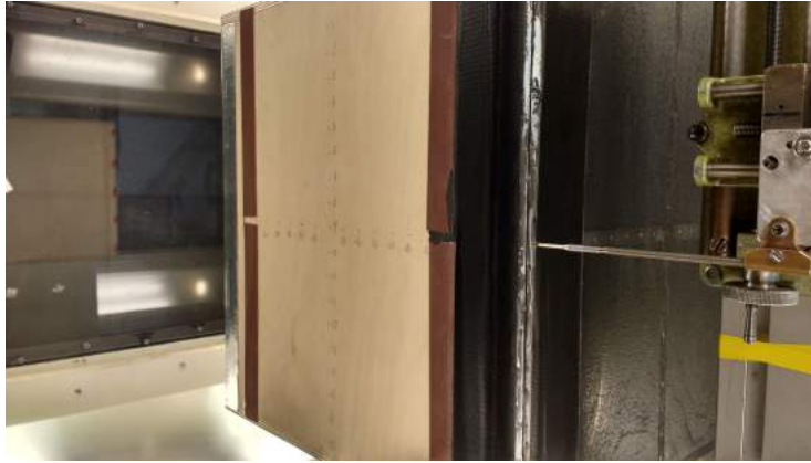
Figure 2.8: The hot wire anemometry setup
