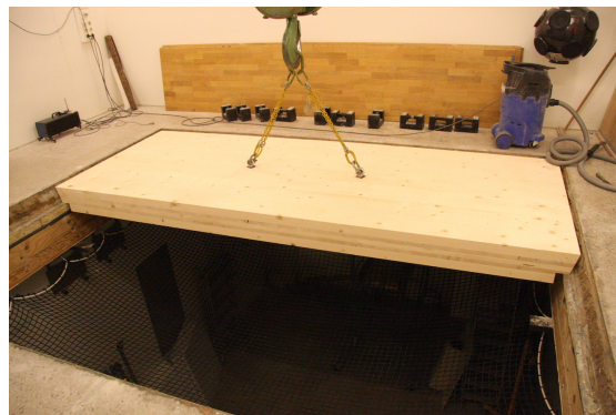
Figure 1. Wooden floor during installation in the lab.
