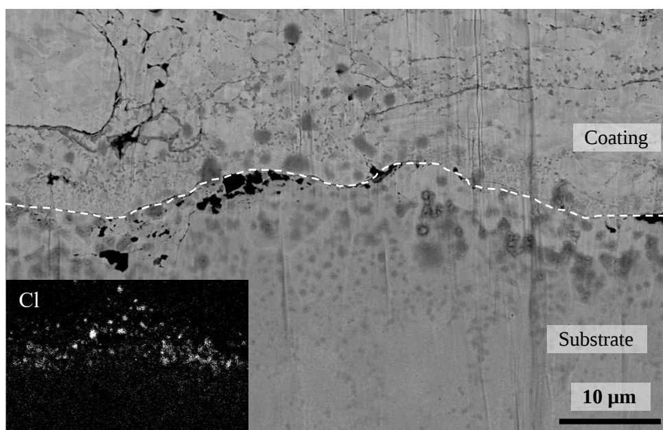
Figure 46: SEM image using BSE of a cross section of the coating/substrate interface of a NiCr-coated sample after exposure in 5% O 2 + 20% H 2 O + N 2 + 1.0 mg/cm 2 at 600 °C for 168 hours. The signal for chlorine from the EDX analysis is located at the bottom left of the picture. The dashed line represents the coating/substrate interface.
