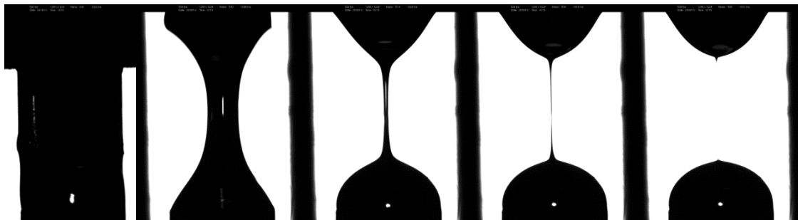
Figure 12: Schematic of filament evolution in the CaBER: (a) loaded; (b) during stretching; (c) shortly after stretching is stopped; (d) during capillary drainage; and (e) after breakup of the Newtonian syrup with 0.55 Pa.s of shear viscosity.
