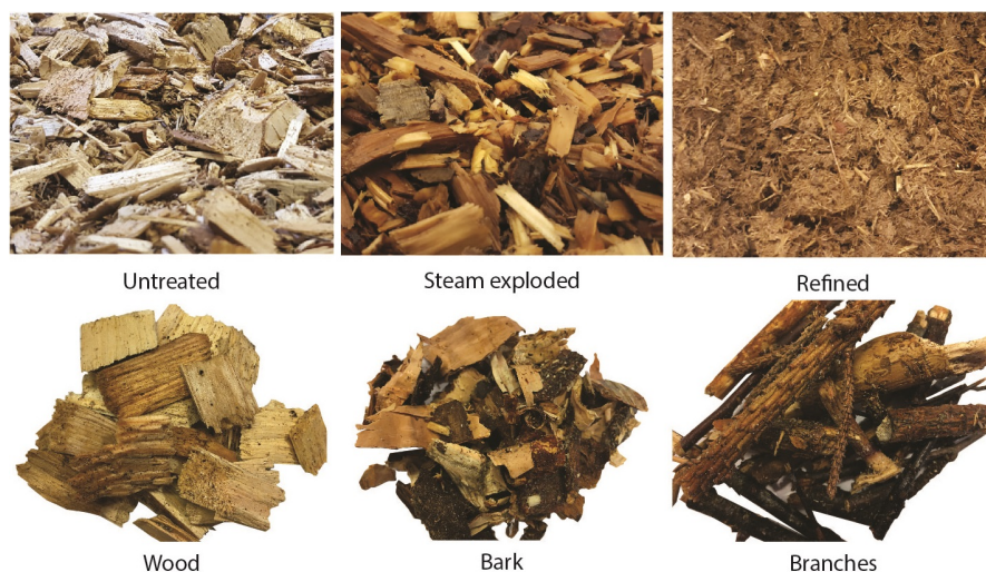
Figure 4.5: The material analysed. Above: untreated, steam exploded and refined forest residues. Below: separated fractions of wood chips, bark and branches.
