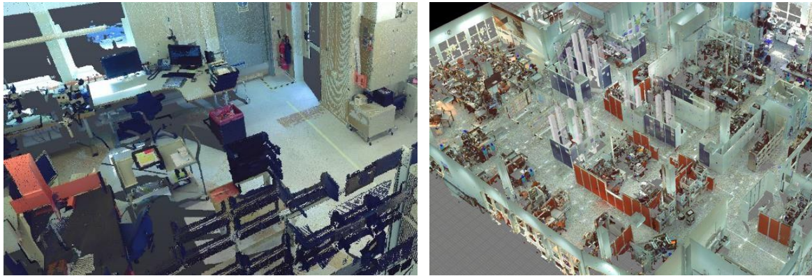
Figure 9. Point cloud of the workshop imported to the simulation software from paper 4
