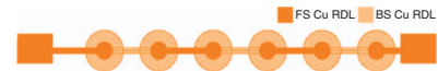
Figure 3 Via daisy chain structure. Two probes land on the probing pads on the left and the right side of the via chain.
