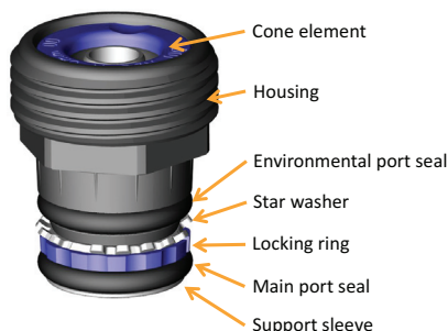
Fig. 1. A KAtridge™ coupling.
