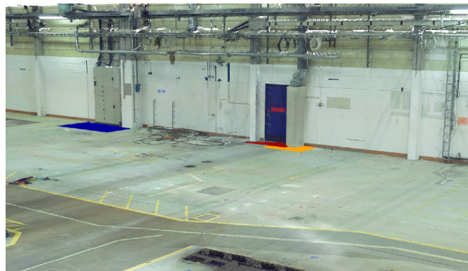
Fig. 1. A workspace visualized by a point cloud where an electric service station (blue), a door (red) and a ventilation shaft (orange) has been modelled as resources that requires regions on the floor to ensure proper functionality and maintenance work. Courtesy by GKN.
