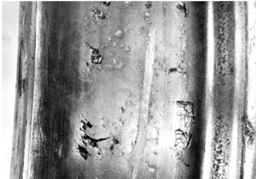
Figure 2.2: Surface damage from surface initiated fatigue. Figure from [24].
