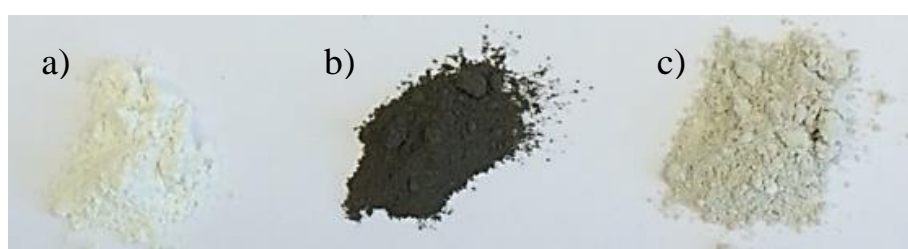
Figure 11: Colour of virgin and recycled pigments where a) mix of virgin pigments corresponding to the one in the pyrolysis ash, b) ground pyrolysis ash from Paint A, c) heat treated (oxidized) pyrolysis ash from Paint A.
