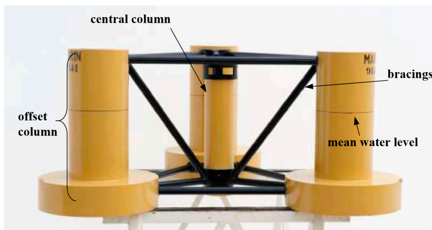
Figure 1. The 1/50 model scale semisubmersible in the DeepCwind tank tests [27,30].
