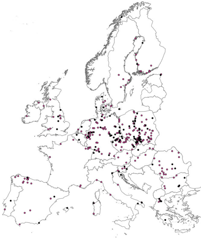
FIGURE 2 Coal-fired power plants included in the CPPD. Black dots: Plants constructed after 1990, for which retrofitting for biomass co-firing is considered economically feasible (Hansson et al., 2009) (142 boilers). Purple dots: Plants that are constructed before 1991 (i.e., assumed to not be available for retrofitting) or have already been retrofitted for co-firing (discussed further in Section 5)
