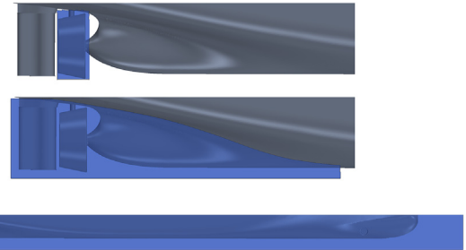
Fig. 5. Alternative control volumes. A) Enclosing the propeller, B) enclosing the aft-ship and C) enclosing the entire vessel.
