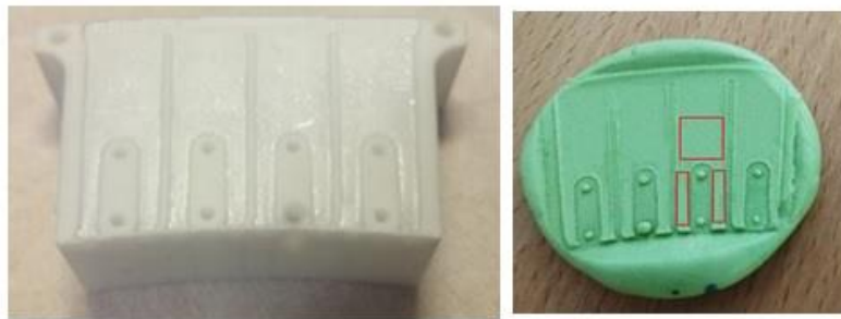
Figure 17. Left: Resulting naphthalene specimen. Right: Imprint taken from a specimen and the 3 areas of interest for scanning.
