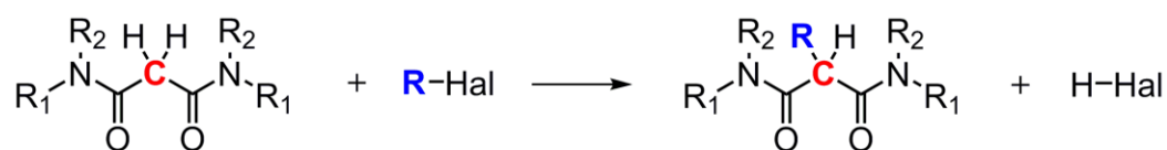
Figure 14 – The scheme of synthesis of the C-alkylated malonamides. R, R 1 and R 2 are alkyl substituents. Hal stands for a halogen atom (Cl or Br).
