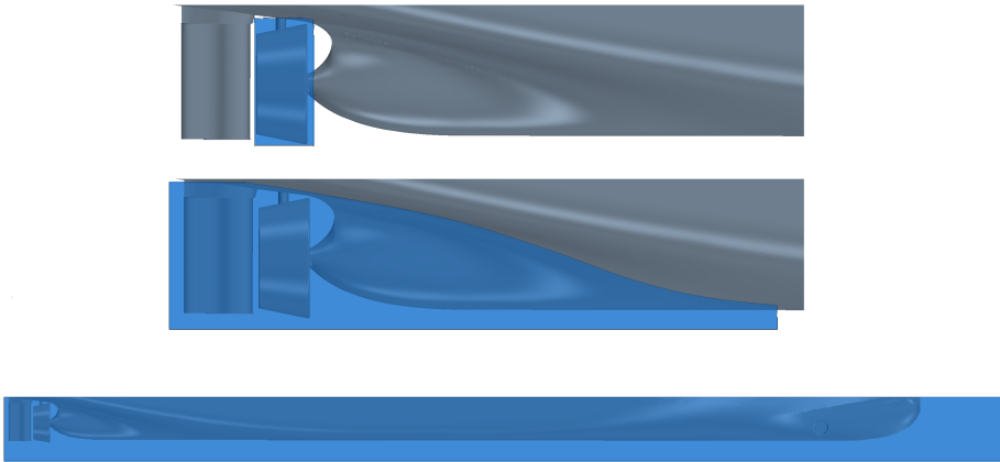
Figure 2.3: Alternative control volumes enclosing: the propeller and duct, the aft-ship and the entire vessel.
