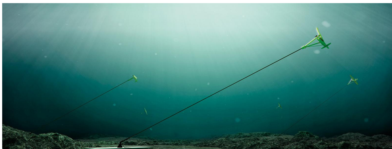
Figure 1. Illustration of the Deep Green tidal current kite concept (Minesto).
