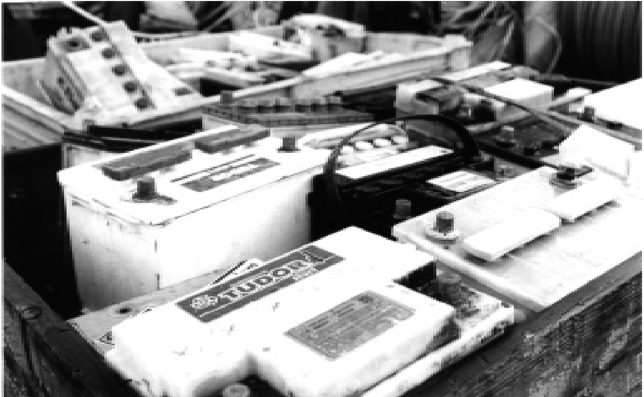
Fig 7.3 Lead in car batteries constitutes a major part of the flow of lead in society. It is comparatively easily subjected to efficient recycling strategies.
