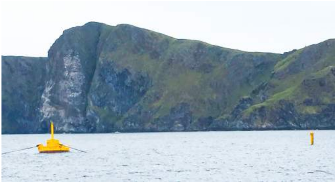
Figure 11. WaveEL 3.0 installation in Runde, Norway. The WEC and two of its mooring legs are shown to the left, and the hub is shown to the right. The power cable between the two is submerged.
