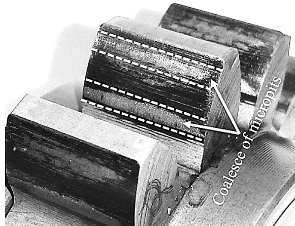
Figure 3. Micropitting on a gear tooth.
