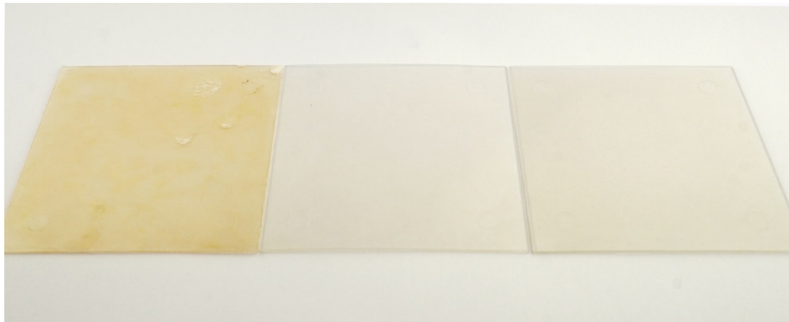
Figure 7: Composites with 10 weight-% CNC, from left; CNC-Morph-OH, CNC-diHexyl-OH and CNC-diAllyl-OH.
