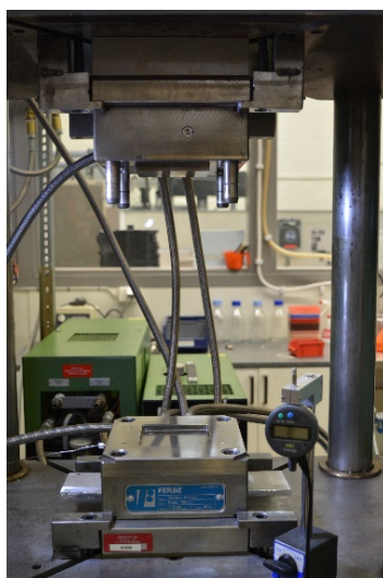
Figure 4: The compression moulding equipment used in the present study.
