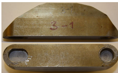
Fig.1. „Side“ (up) and „bottom“ (down) view of the valve bridge component prototype for heavy duty engine application.
