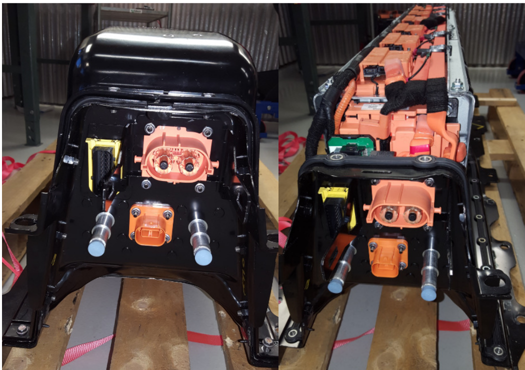
Figure 9.9 - Inert battery pack. The side with the CIDD (upper) and HVCH (lower) connector. With and without lid
