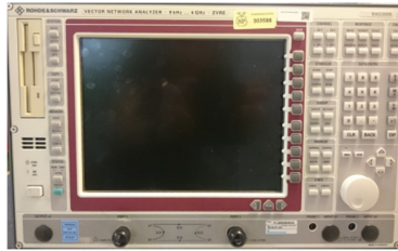
Figure 8.26 - Network analyzer ZVRE for measuring S-parameters.
