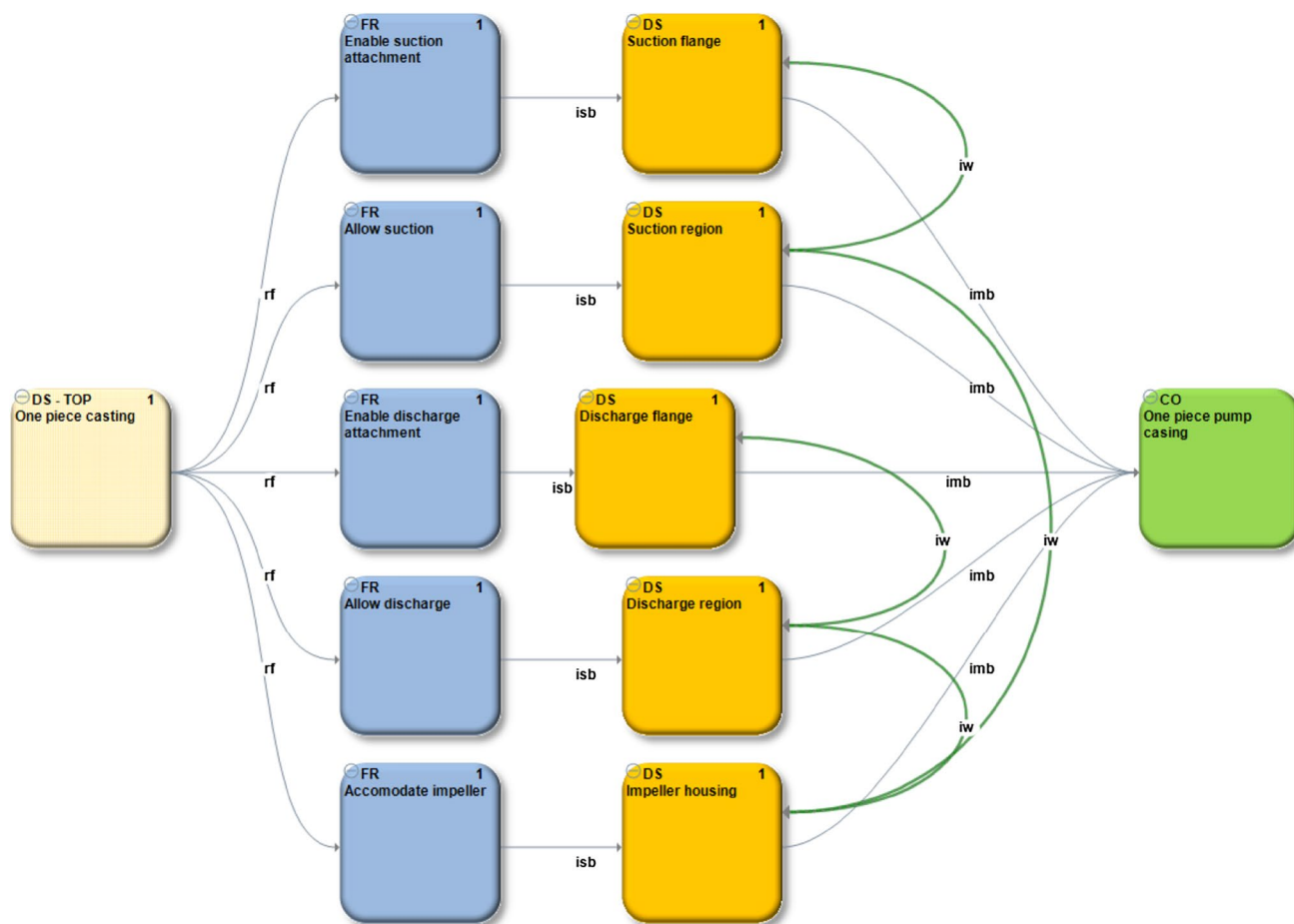
Fig. 11 EF-M tree for the cast pump casing design (as generated in the CCM tool)
